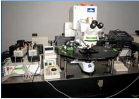
Multiphoton excitation confocal microscope. This is a Zeiss LSM510 NLO.
